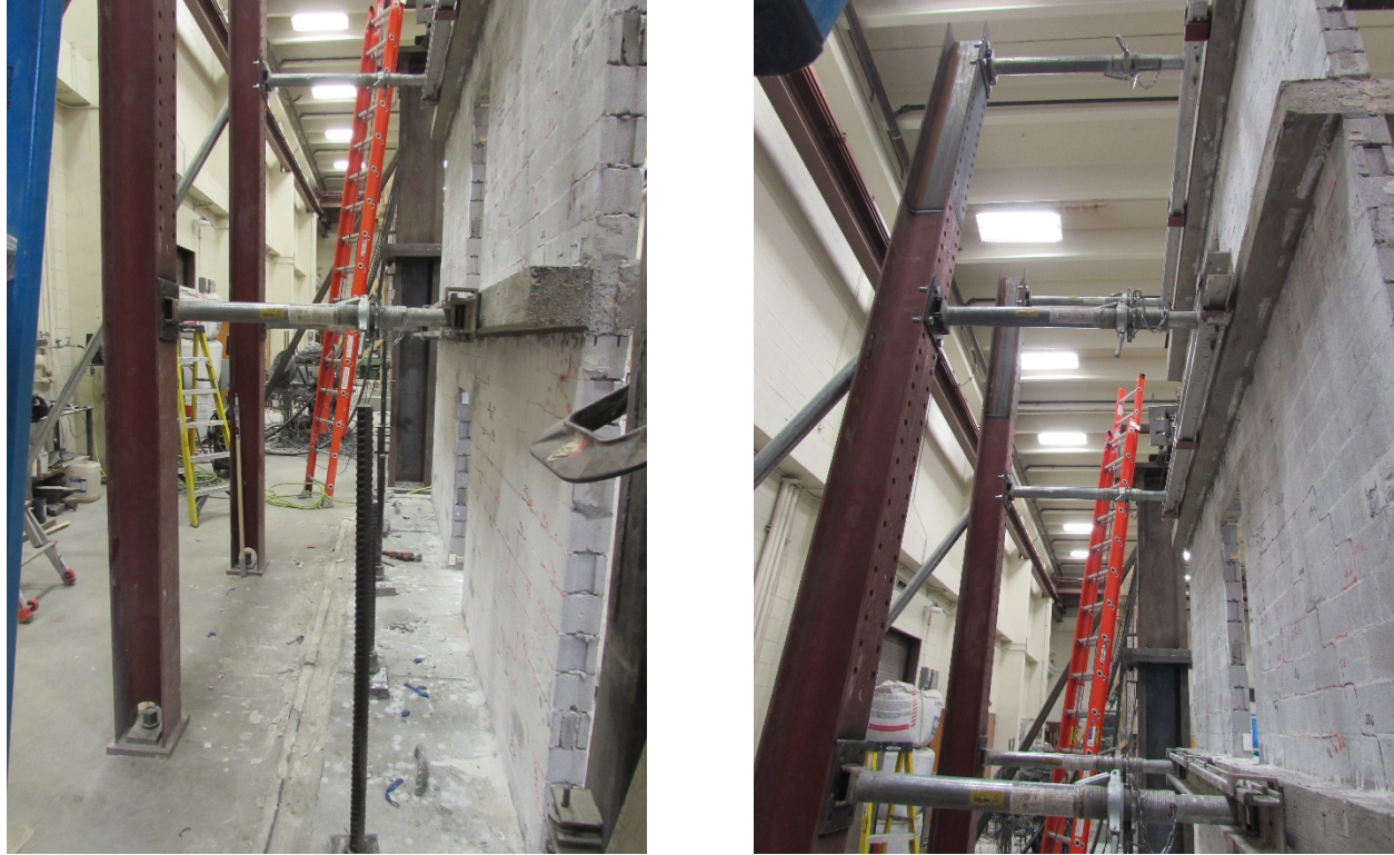
Figure 3-7: Out-of-Plane Bracing System
