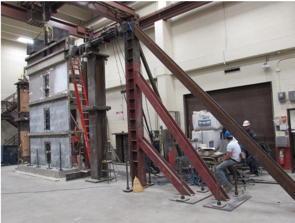
Figure 3-6: Wall Testing Apparatus
