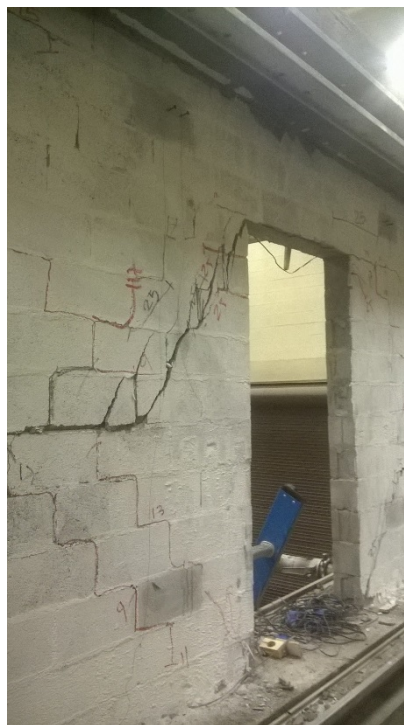
Figure 3-12: Marking Cracks During Testing
