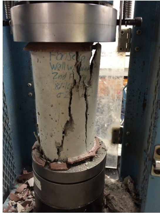
Figure B-4: Testing of Concrete Cylinder
